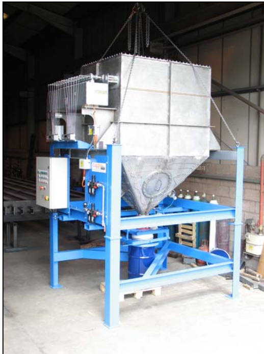
Caldo ceramic filter for fuel gas filtration at 700°C. The filter is built in type 304 stainless steel and incorporates trace heating and a metal seated solids discharge ball valve
